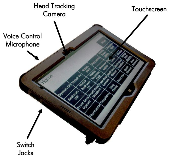
All of these access methods can be used simultaneously to provide the best ease-of-use experience available anywhere.
